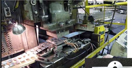
**BLANKING-** Using a compound die to blank and pierce coiled material we create this "two-off" pierced blank.
