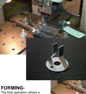
The final operation utilizes a "stock tool" to form the final bend (two hits) creating the finished part.
